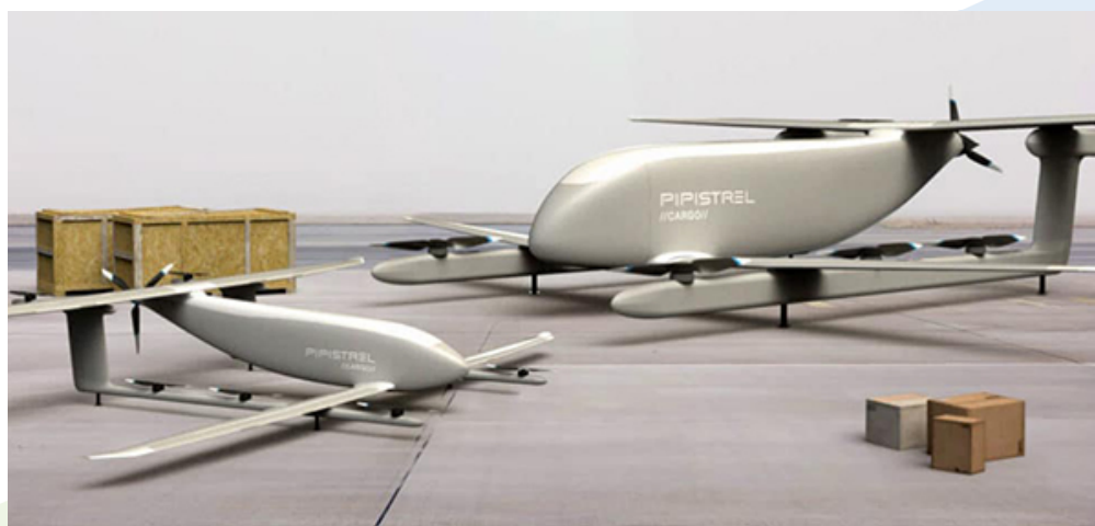
Figure 3-2. Conceptual Drawing of Pipistrel's Cargo eVTOL (GPS World, 2020)
